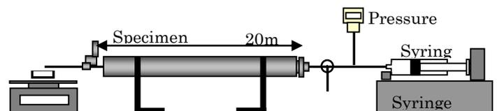
Fig.1 Schematic of injection apparatus
