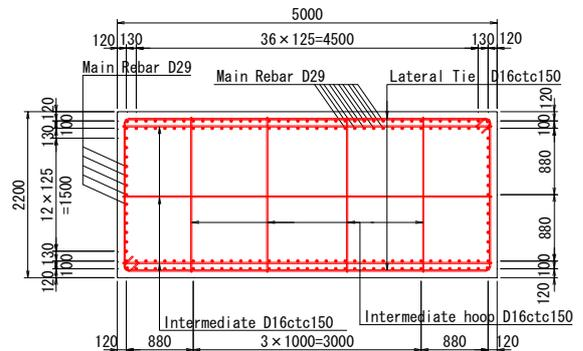
Fig. 4: Rebar Arrangement of the Pier Column
