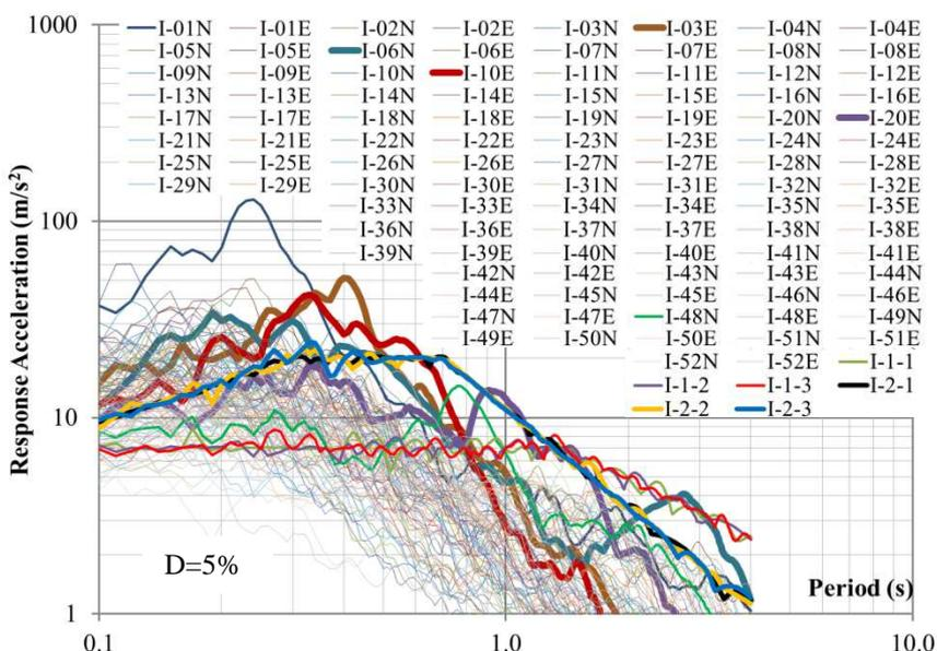
Fig. 1: Response Acceleration Spectrum of Main Ground Motions
