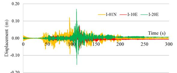
Fig. 5: Response Displacement of Superstructure
