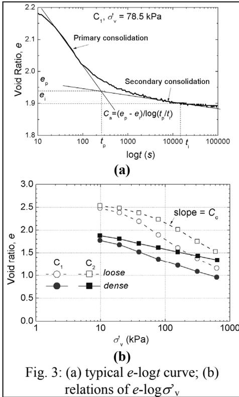
Fig. 3: (a) typical  $e$ - $\log t$  curve; (b) relations of  $e$ - $\log \sigma'_v$
