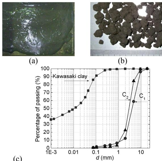
Fig. 1. (a) Kawasaki clay; (b) CTGS ( $C_1$  type) and (c) grading curves of the materials
