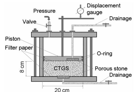
Fig.2. the model of one-dimensional consolidation test
