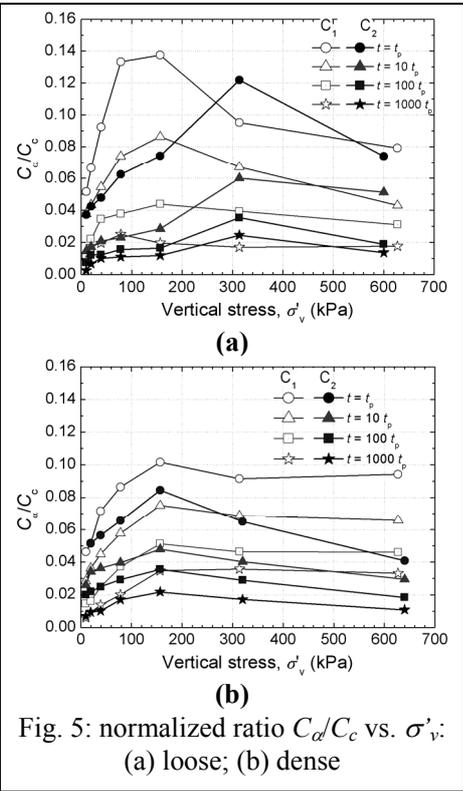
Fig. 5: normalized ratio  $C_d/C_c$  vs.  $\sigma'_v$ : (a) loose; (b) dense
