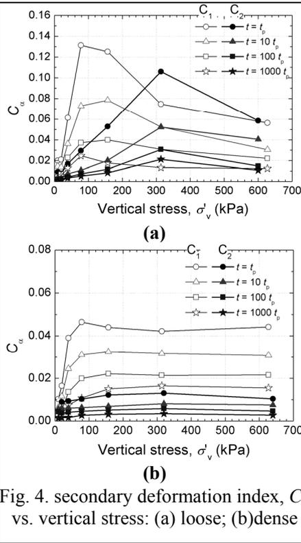
Fig. 4. secondary deformation index,  $C_\alpha$  vs. vertical stress: (a) loose; (b) dense
