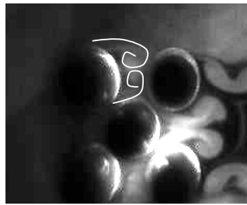
Figure 5 Angle of attack =0[deg.], Flowfield of aerodynamic force peak
