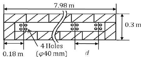
**Fig. 2** Double wythes clay brick masonry wall with grouted cavity (not to scale).
