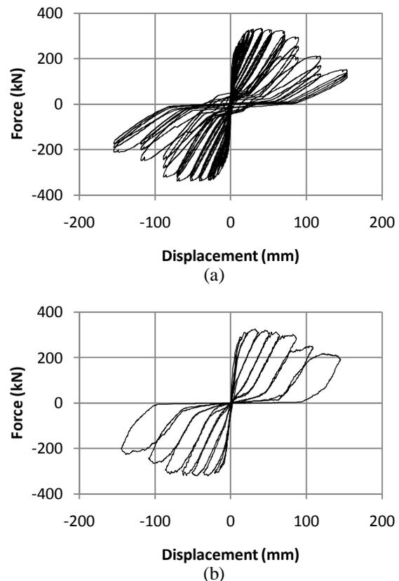
**Fig. 1** Force-displacement history: (a) experiment; (b) FEM.
