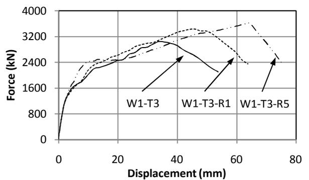
**Fig. 4** Force-displacement curves for W1-T3 with different reinforcement ratios.
