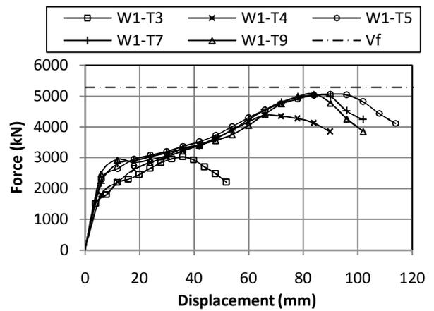
**Fig. 3** Force-displacement curves for different tendon spacing.
