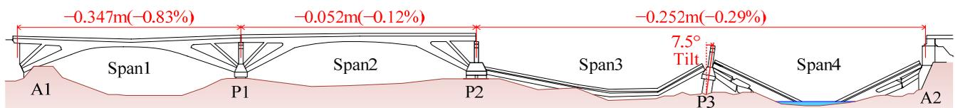
Fig.1 Overall Failure of Xiaoyudong Bridge (from upstream)
