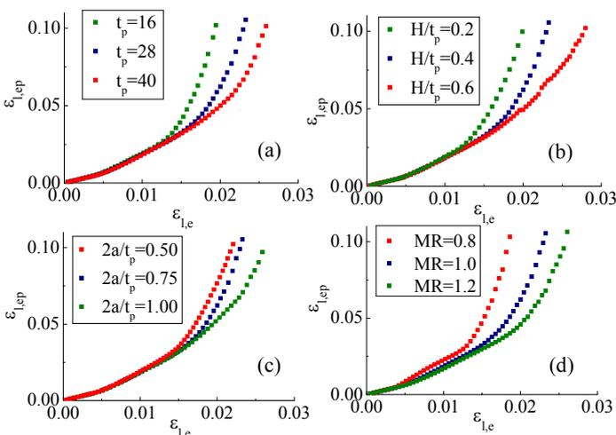
**Fig. 3** Effect of plate thickness(a) weld leg(b) incomplete penetration (c) and Material matching (d)
