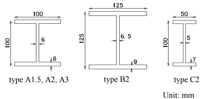
Fig. 1 Details of sections of H-beams
