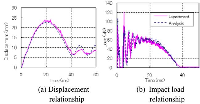
Fig. 4 Time responses of displacement and impact load at midspan for beam type A2,  $V_{col}=2$  m/s.
