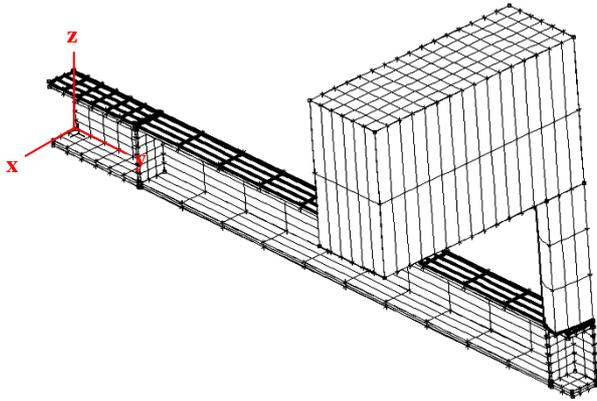
Fig. 3 Finite element model of quarter part
