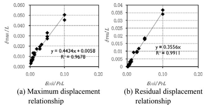
Fig. 5 Relationship between the displacement-span length ratios  $\delta/L$  to kinetic energy-yield bending capacity  $E_{col}/P_yL$ .
