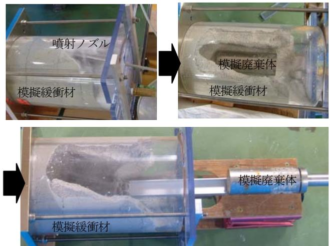
図1 塩水噴射による緩衝材除去実験例<sup>2)</sup>
