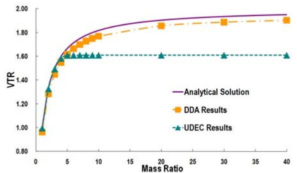
Figure 5 VTR versus MR of DDA and UDEC, E  $10^{13}$ pa, P  $10^9$ N/m
