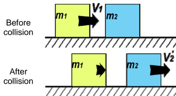
Figure 1 Collision blocks with no friction
