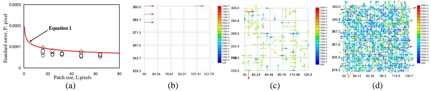
**Fig.3** PIV precision validation: (a) Measurement standard error against patch size; Example results for scatter of displacement vectors (in mm) for 32 pixels search zone and zero incremental displacement for patch sizes of (b) 64x64, (c) 32x32 and (d) 16x16 pixels.
