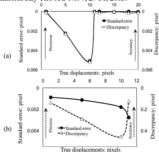
**Fig.4** Movement accuracy results: (a) image-shifted displacements, (b) micrometer-driven displacements
