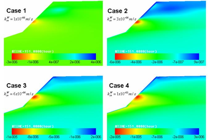
Fig. 3 Horizontal water velocity (m/s) at t=151 h.
