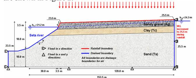
Fig. 1 Cross section of embankment and boundary conditions
