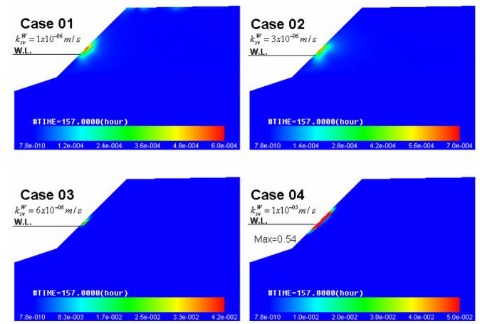
Fig. 4 Viscoplastic shear strain at t=151 h.
