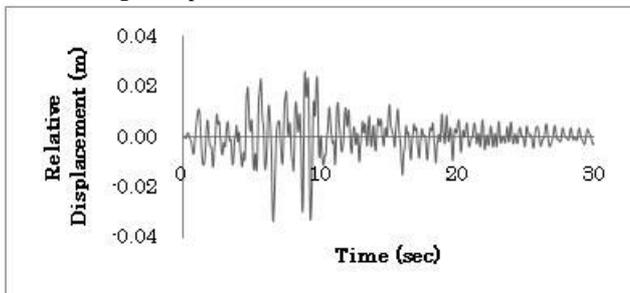
**Fig 5** Displacements at the end of abutments
