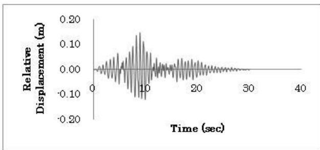
**Fig 3** Displacements at the end of abutments
