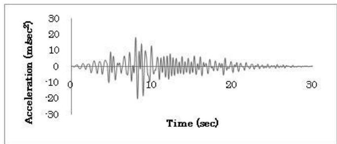
**Fig 4** Accelerations at the center section of the bridge
