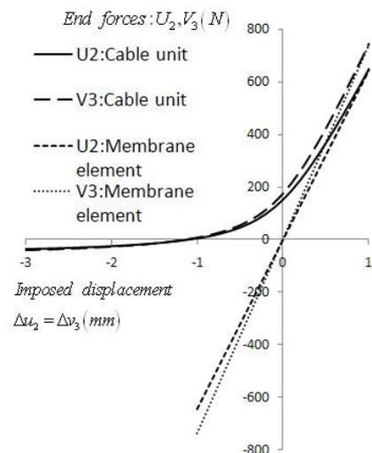
Figure5: Comparison between cable unit and membrane element
