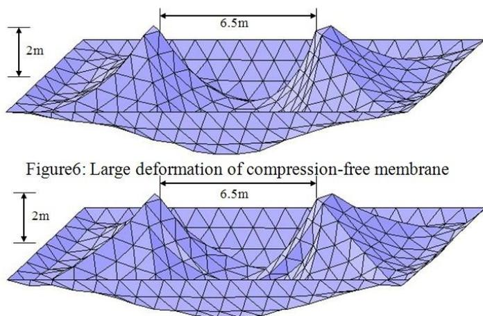
Figure7: Large deformation of membrane considering compressive stiffness
