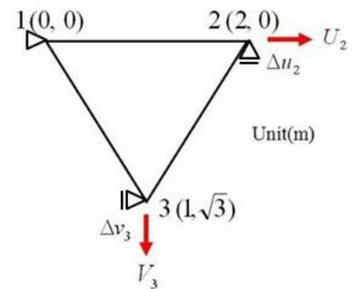
Figure4:Cable unit element of equilateral triangle
