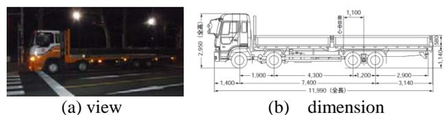
**Fig.3** – 25-ton test truck
