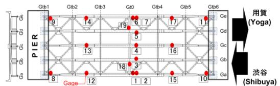
**Fig.2** – Location of strain gauges over each span
