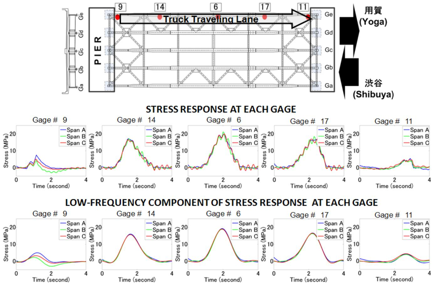
Fig.4 – Stress responses of main girder Ge (truck ran at Yoga-bound, outer/slow lane, with speed = 60 km/h)
