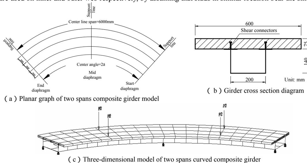
Fig.1 Detailed Geometry of Girder Model
