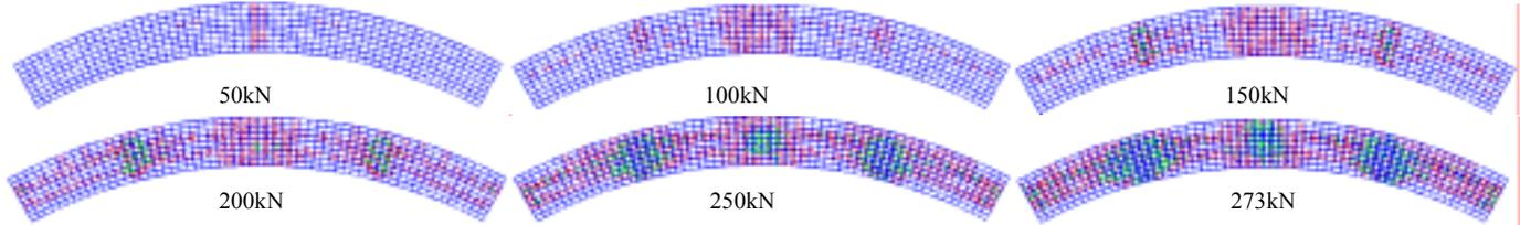
Fig.4 Cracking development process of concrete deck
