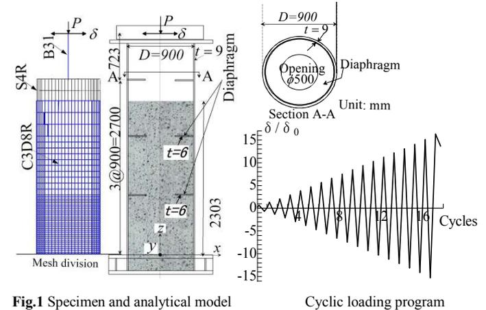
Fig.1 Specimen and analytical model
