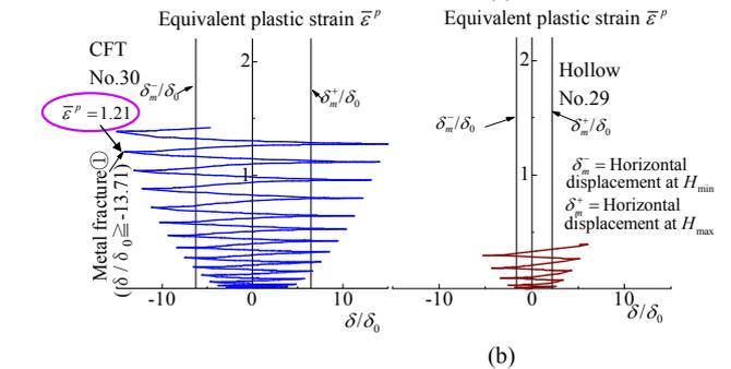
Fig.8 (a) Location of metal fracture (No.30), (b) Fracture initiation criterion
