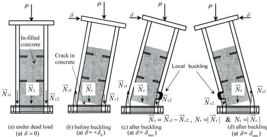
Fig.6 Resisting mechanism of CFT column
