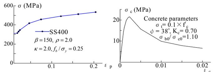
Fig.2 Uniaxial stress-strain relation of steel
