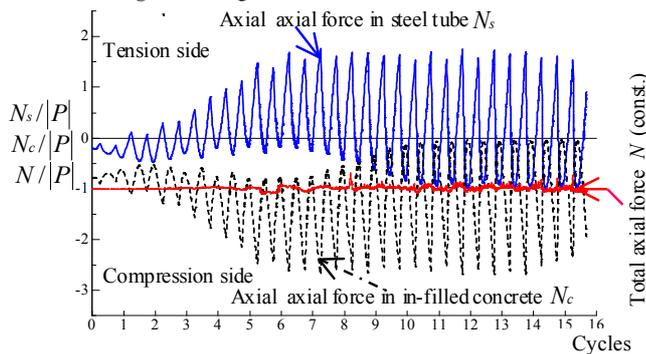
Fig.7 Axial load distribution in steel tube and in-filled concrete (No.30)
