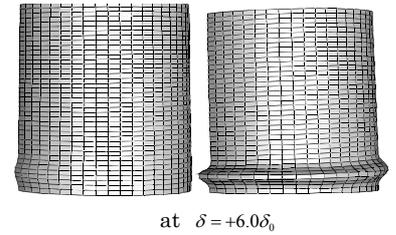
Fig.5 Deformed shapes at the lower part of steel pipe (x1.5)
