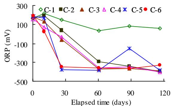
Fig. 5. ORP value in pore water at P-4 segment
