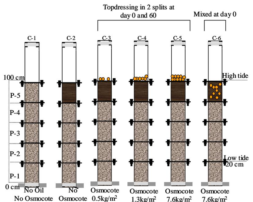
Fig. 1. Sand columns imposed with treatments
