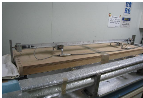
Figure 2 Installation of displacement transducers after 24 hours
