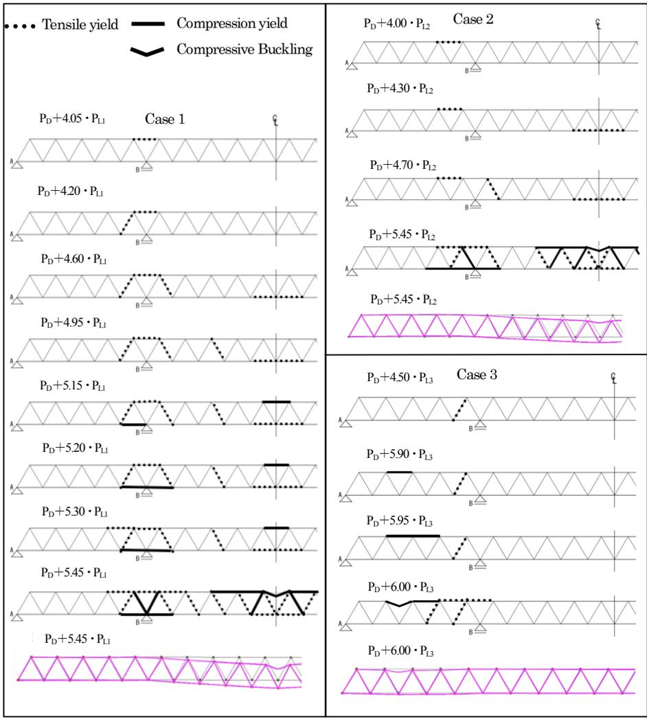
Fig.6 Collapse Process and Final Deformation
