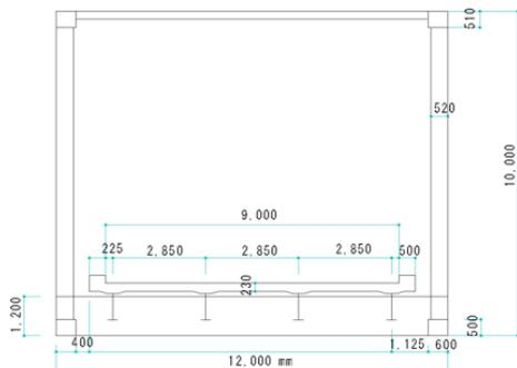
Fig.2 Cross-Section (mm)
