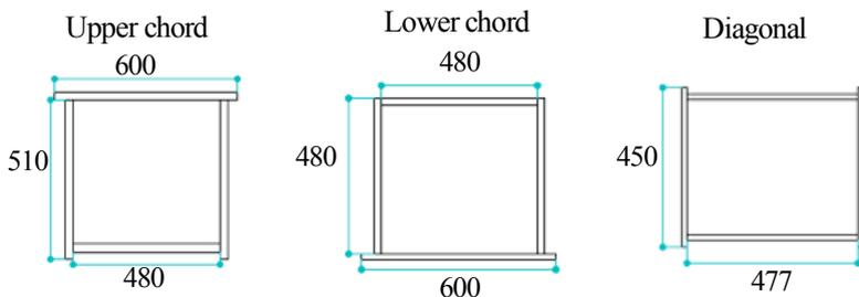
Fig.4 Cross-Section of Structural Members (mm)
