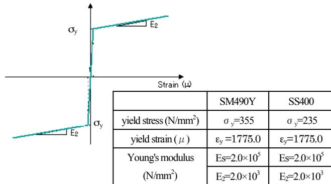
Fig.3 Stress-Strain Curve of Steel
