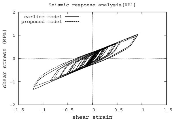
Fig. 6. Results of seismic response analysis using RB1
