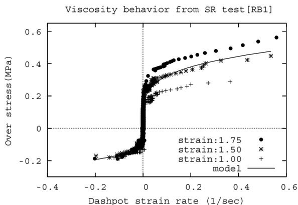
Fig. 1. Typical rate dependent overstress of RB1
