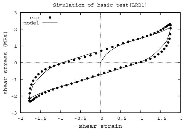
Fig. 5. Simulation results of LRB1
