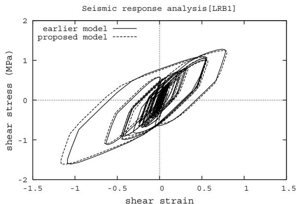
Fig. 7. Results of seismic response analysis using LRB1
