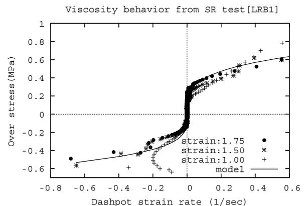
Fig. 2. Typical rate dependent overstress of LRB1
