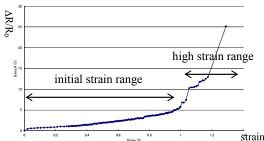
Fig. 1  $\Delta R/R_0$  vs.  $\epsilon$  of CFS
