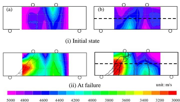
**Fig. 4: 2-dimensional velocity structures of central cross section for a) plain concrete specimen and b) composite specimen**
