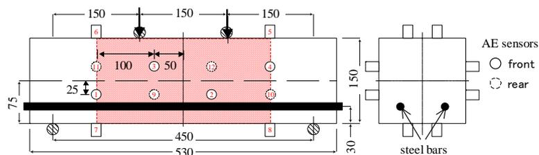
Fig. 1: Specimen and AE sensors arrangement (unit: mm)
