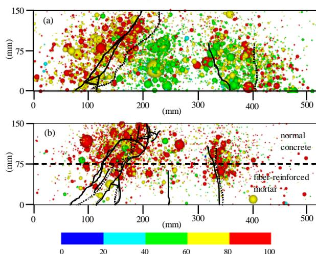
**Fig. 3: Locations of AE events and actual cracking patterns for a) plain concrete specimen and b) composite specimen (solid line: crack from front view, dash line: rear view)**
