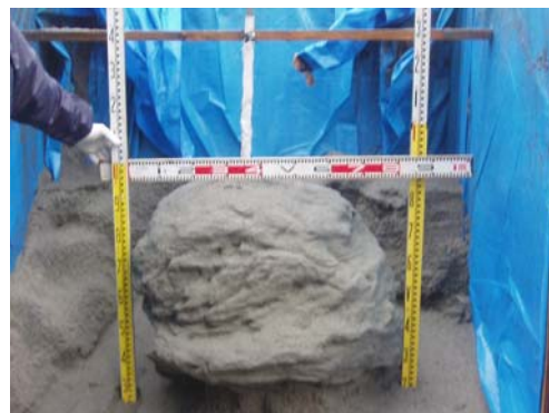
写真-2 改良体全景 (500%)
