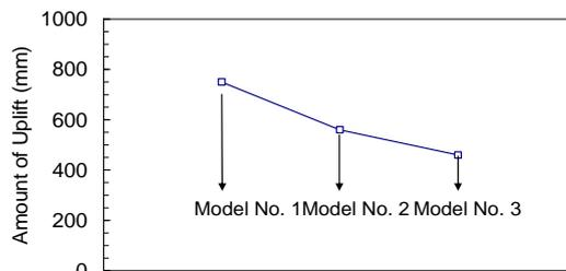
Fig. 7. Amount of uplift of manholes
