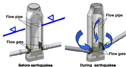
Fig.1. Flow gates and flow pipe as countermeasure
