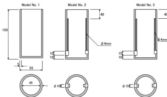
Fig. 3. Manhole model and countermeasures
