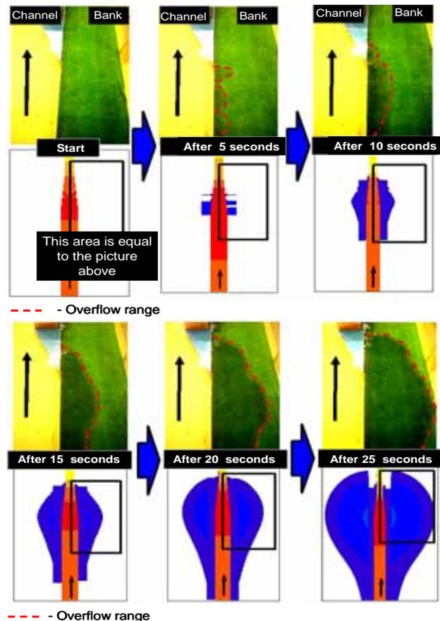
Figure 5: Inundation Results (0-25seconds)
