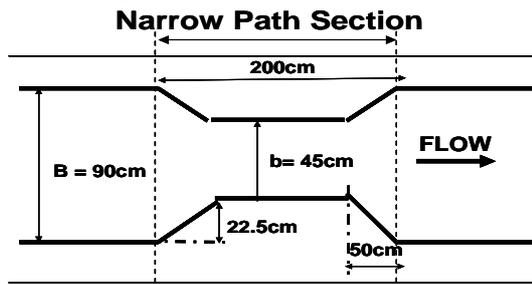
**Figure 1:** Small-scale Narrow Path River Model Detail
