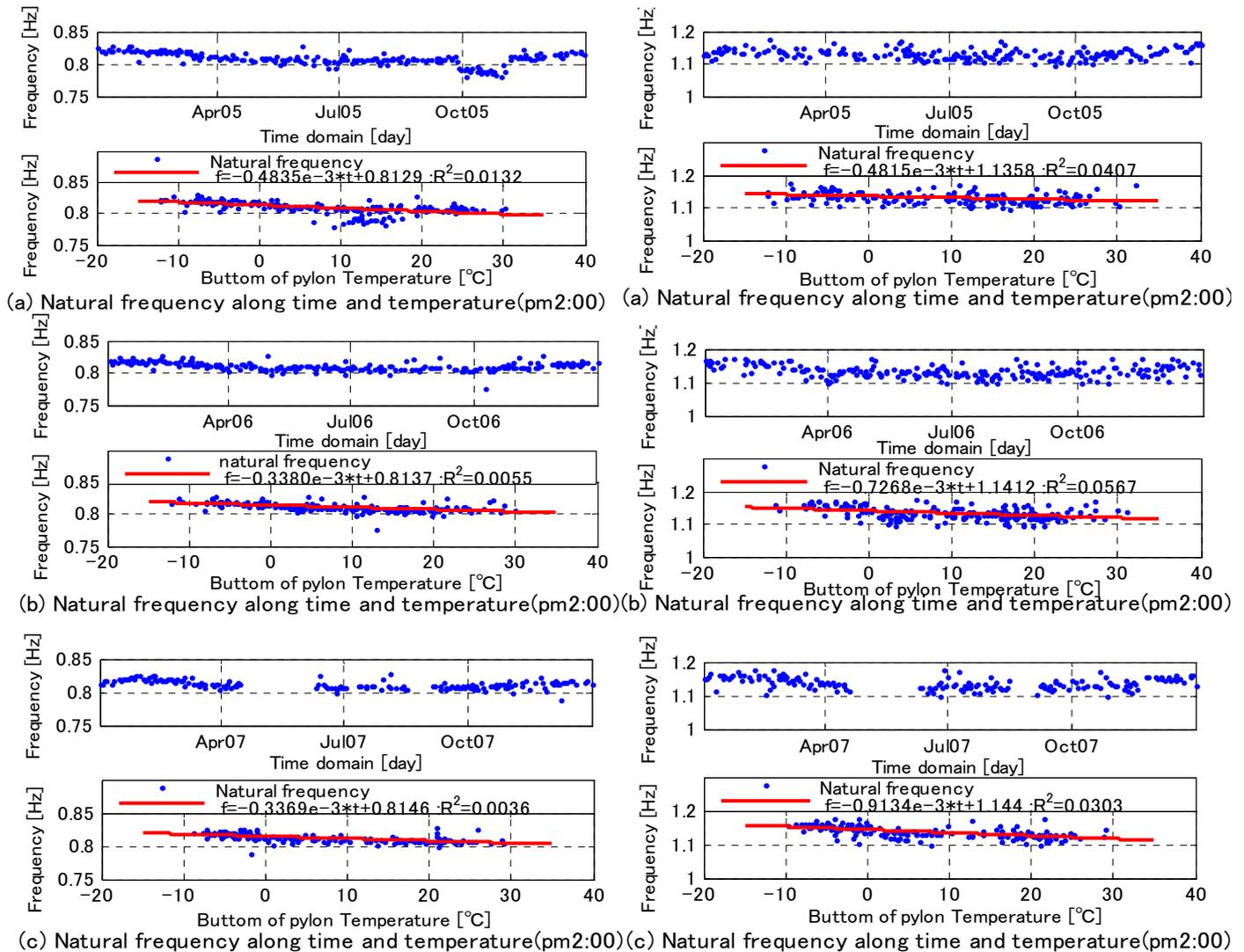
Fig. 2 Fluctuation of the 2<sup>nd</sup> mode natural frequencyFig. 3 Fluctuation of the 3<sup>rd</sup> mode natural frequency
