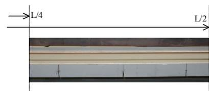
Fig. 2 Damaged girder with saw-cuts
