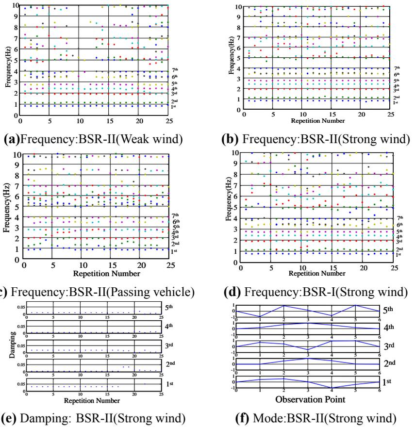
**Fig.5** Estimated dynamic characteristics Figures 5(a), 5(b), and 5(c) are the graphical representation of estimated frequency by BSR-II method for weak wind, strong wind and passing vehicle respectively. Fig 5(a) shows the steady estimation upto 5<sup>th</sup> mode, Fig.5(b) shows the steady estimation up to 7<sup>th</sup> mode frequency whereas Fig.5(c) shows the
