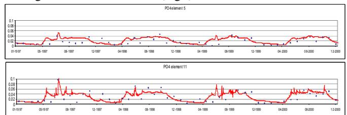
Fig. 7 PO<sub>4</sub> concentration (mg/l) in element 5 and element 11
