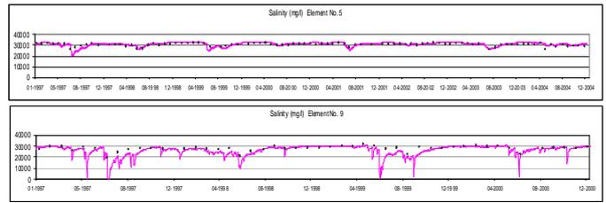
Fig. 2 Salinity concentration (mg/l) in element 5 and 9
