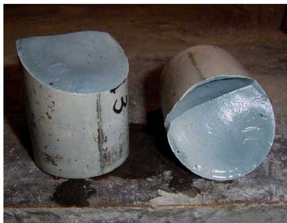
Photo 1 Cement paste broken by sodium
