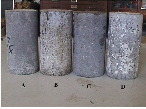
**Fig. 1. Surface deterioration of Concrete samples After Exposure to Wet-Dry Cycles**
