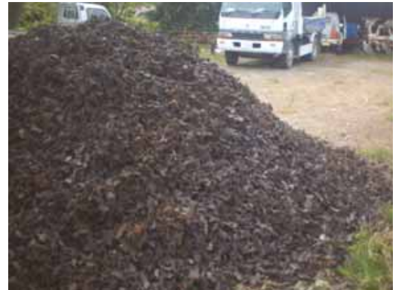
Fig.4 Scrap tire shreds used for backfill.
