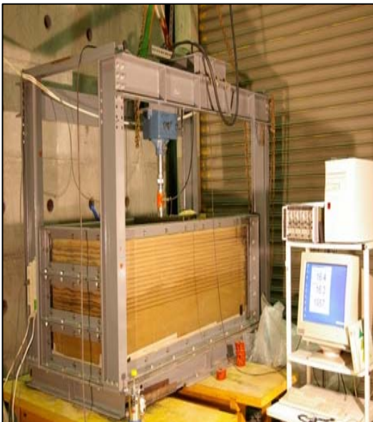
Figure.1. General view of experimental set-up for model-scale footing tests
