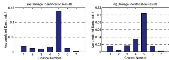
Fig. 2 Damage identification results for damage location at N5 using experimental data obtained from test 1 and test 2
