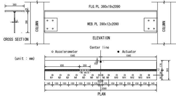
Fig. 1 Beam layout, main dimensions and sensor locations
