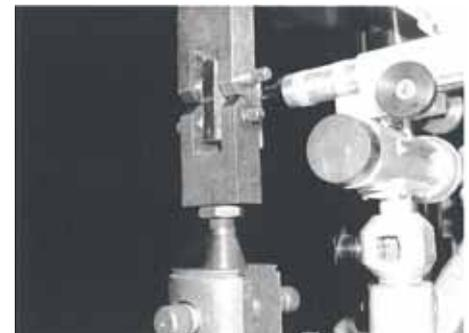
Picture 1 Installation for fatigue tests with crack length monitor
