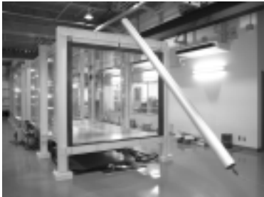
Fig.3 Set up for the cable model ( \alpha=-45^\circ , \beta=90^\circ )
