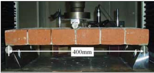
Figure 3 Out-of-plane test setup
