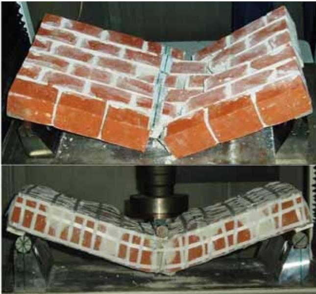
Figure 4 Failure patterns of brick masonry wallettes without and with retrofiting
