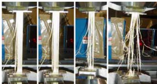
Figure 2 Failure pattern of PP-band under tensile force
