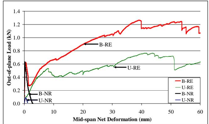
Figure 5 Out-of-plane load variations in terms of net vertical deformation
