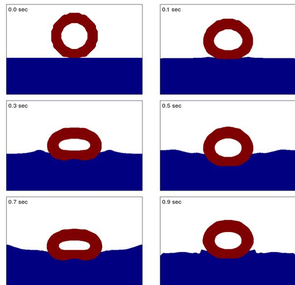
**Figure2** Computational result of ring falling onto fluid
