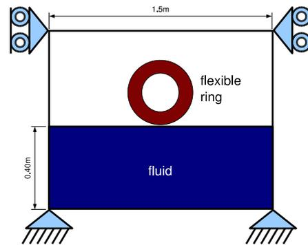
**Figure1** Ring Falling onto Fluid
