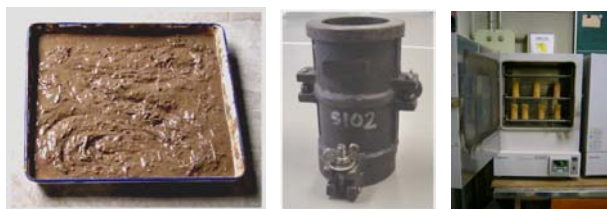
Fig. 1. Preparation of adobe specimens
