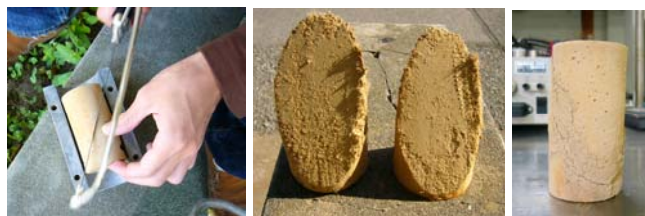
Fig. 6. Preparation of sandwich specimens
