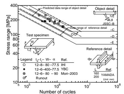
Fig 3: Predicted S-N diagram and fatigue test data
