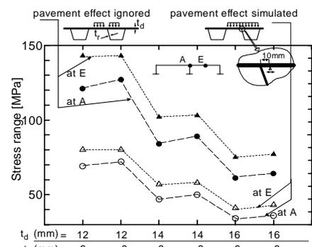
Fig 5: Stress ranges from various two-panel deck models
