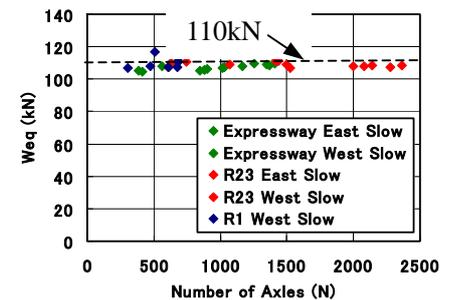
Fig 6: Equivalent axle load from actual measurement in Nagoya
