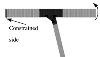
Fig 2: A FE model used for fatigue life prediction
