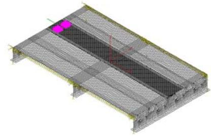
Fig 4: Two-panel deck model
