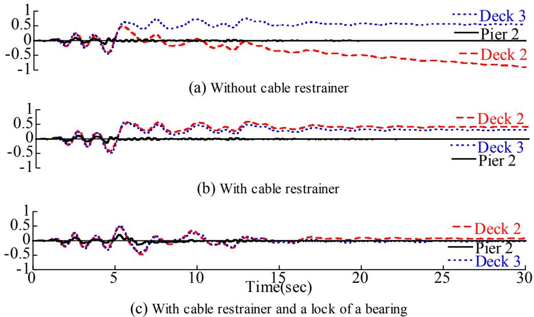
Fig. 4 Comparison of response displacement of the Deck2, Deck3 and Pier2
