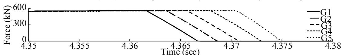
Fig. 3 Progressive failure of bearings which support Deck 3 on Pier 2
