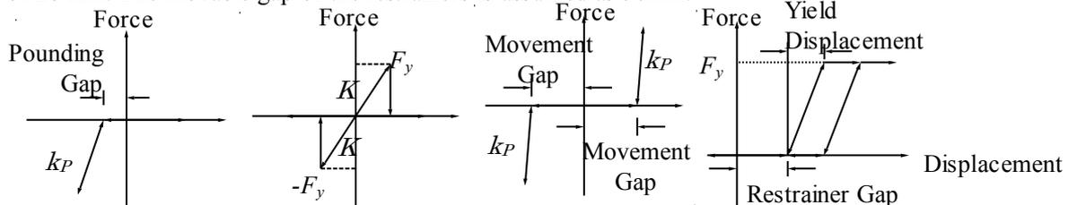
Fig. 2 Idealization of pounding, bearing and cable restrainer
