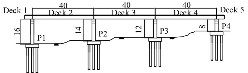
Fig. 1 Target bridge (unit in meter)
