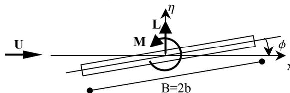
Fig. 2 Definition of motion and force components
