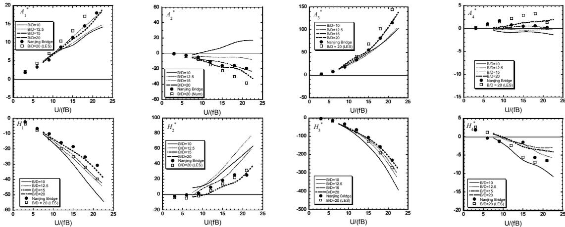
Fig. 3 Comparison of aerodynamic coefficients of Rectangular Section ( $B/D=20$ ) and Nanjing Bridge Section ( $B/D=11.6$ ) with the experimental results of different  $B/D$  ratios<sup>3</sup>
