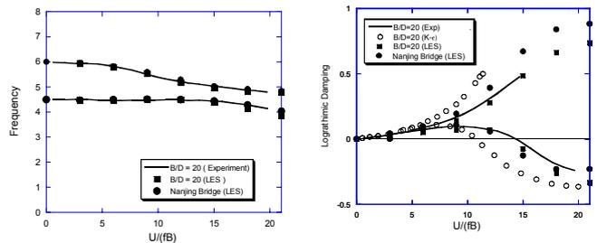
Figure 4 Eigen value loci of Rectangular cross section and Nanjing Bridge.  $M=1.96kg/m, I=4.9 \times 10^{-3} Kg m, f_{\theta 0}=4.5 Hz, f_{\theta 0}=6.0 Hz, B(=2b)=0.15m$
