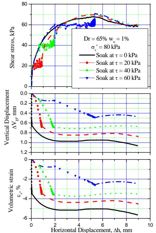
Fig. 4 The relationships on effect of shear level of infiltration process of a)  $\tau$ - $\Delta h$ , b)  $\Delta V_D$ - $\Delta h$ , c)  $-(\Delta V_D/V_{D0})$ - $\Delta h$
