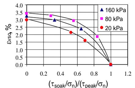
Fig. 5 Relationship between  $\epsilon_{vs}$  during soaking and normalized shear stress level  $(\tau_{soak}/\sigma_n)/(\tau_{peak}/\sigma_n)$  at soaking
