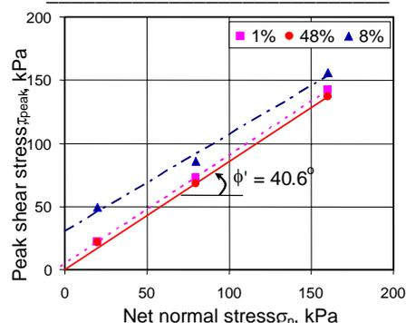
Fig.1 Relationship between net normal stress and strength for compacted specimens with  $Dr = 65\%$
