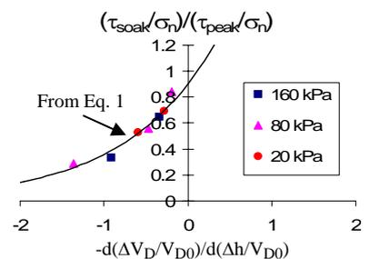
Fig. 6 Relationship during soaking process between  $(\tau_{soak}/\sigma_n)/(\tau_{peak}/\sigma_n)$  and  $-d(\Delta V_D/V_{D0})/d(\Delta h/\Delta V_{D0})$
