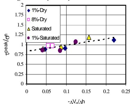
Fig. 2 Relationship between dilatancy index and normalized peak strength under various water contents and confining pressures
