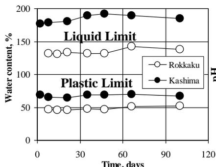
Fig. 3 Atterberg's limits of disturbed samples
