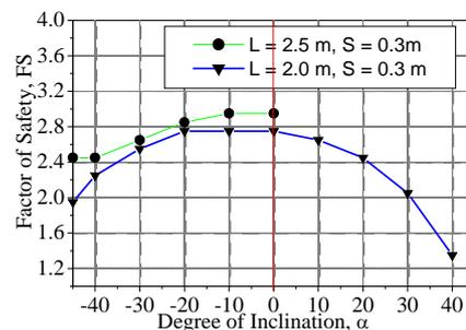
Fig. 8 FS vs. Inclination angle of pile
