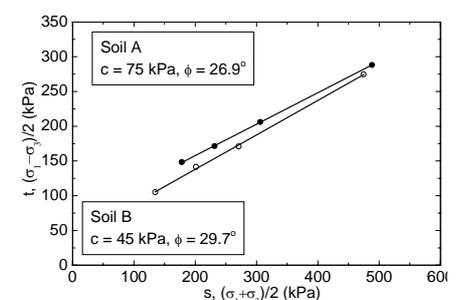
Fig. 3 Failure envelop of total stress on  $t$ - $s$  stress field for Soil A and Soil B
