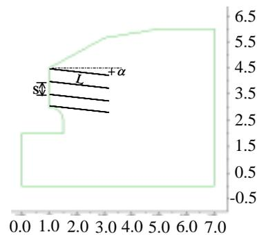
Fig. 5 Sketch of the reinforcement Design for Cave-type of geometry
