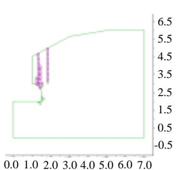
Fig. 4 Tensile failure for Cave-type of geometry ( $FS = 1.45$ )
