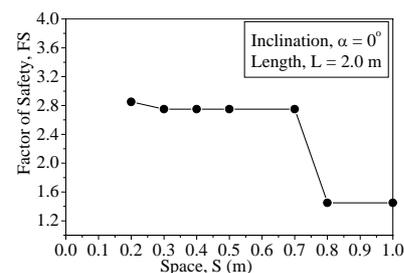
Fig. 7 FS vs. Spacing of pile
