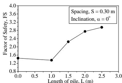
Fig. 6 FS vs. length of pile
