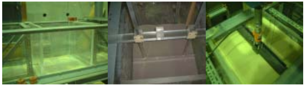
Fig.2: The soil container and the other Mechanical used for model testing of footings.
