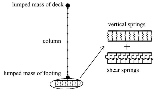
Fig.4 Model used for the analysis
