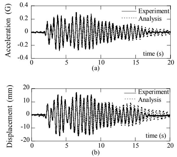
Fig.2 Correlation on the experimental response under 10% JMA Kobe record: (a) horizontal deck acceleration and (b) horizontal deck displacement
