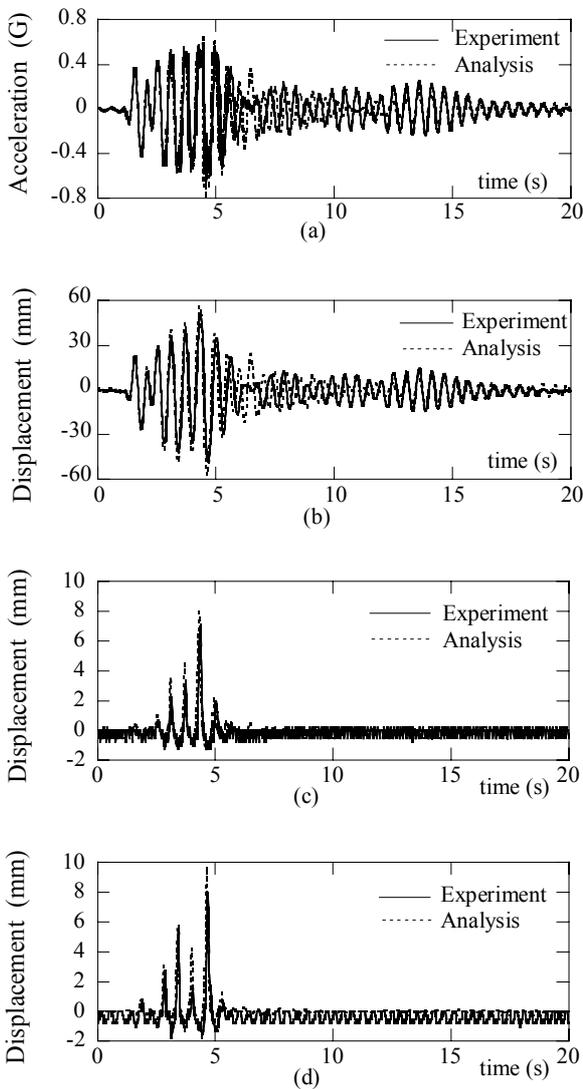
Fig.3 Correlation on experimental response under 25% JMA Kobe record: (a) horizontal deck acceleration, (b) horizontal deck displacement, (c) vertical footing displacement at the left edge and (d) vertical footing displacement at the right edge
