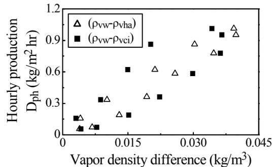
Fig. 4 Relationship between  $D_{ph}$  and vapor density difference
