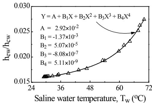
Fig. 2 Variation of  $h_{ew}/h_{cw}$  with  $T_w$
