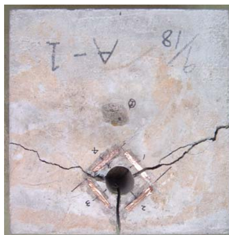
Fig.5 Photograph of crack propagation (left) and SiGMA analysis visualised results (right) of the specimen A.
